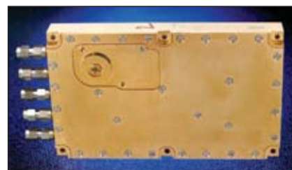
▲ Fig. 11 Farran's five-channel 35 GHz transceiver MMIC module with integrated PLDRO (75 x 125 x 25 mm).
