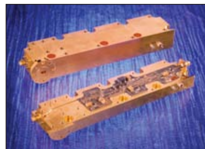
▲ Fig. 6 44 GHz MMIC upconverter module (courtesy of Farran Technology Ltd.).
