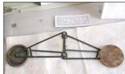
▲ Fig. 4 Apparatus used by Maxwell to determine the speed of light based on electrostatics and magnetostatics.
