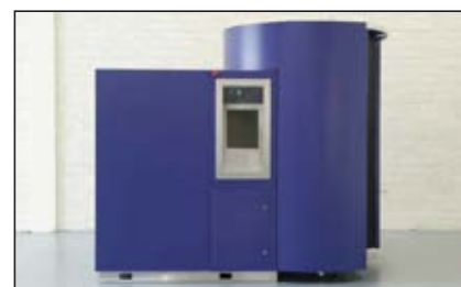
▲ Fig. 9 Millimeter-wave passive imaging camera for portal security. 17
